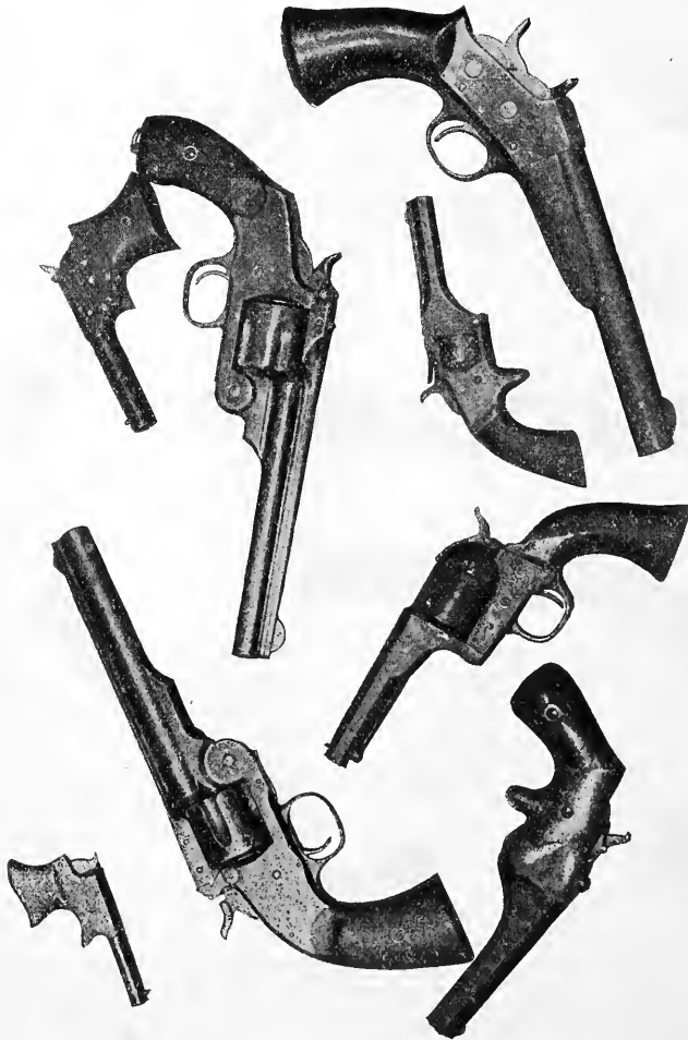
Group of American cartridge pistols from the collection of John Paul Bocock, showing: A, the earliest type of Smith & Wesson revolver; B, the Schofield Smith & Wesson; C, the "Spanish" Smith & Wesson; D, the Hammond bulldog; E, the Remington single-shot army pistol; F and G, Remington derringers.
